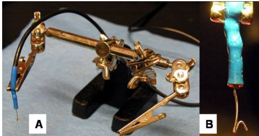
Figure 20 Cathode Stimulator Held By Manipulator
